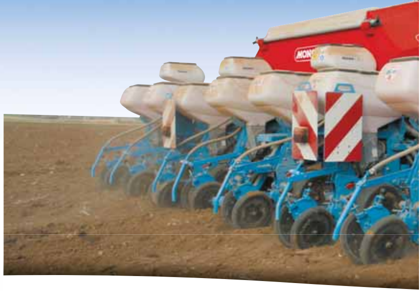
8-row TFC folding planter (75 cm inter row spacing)
