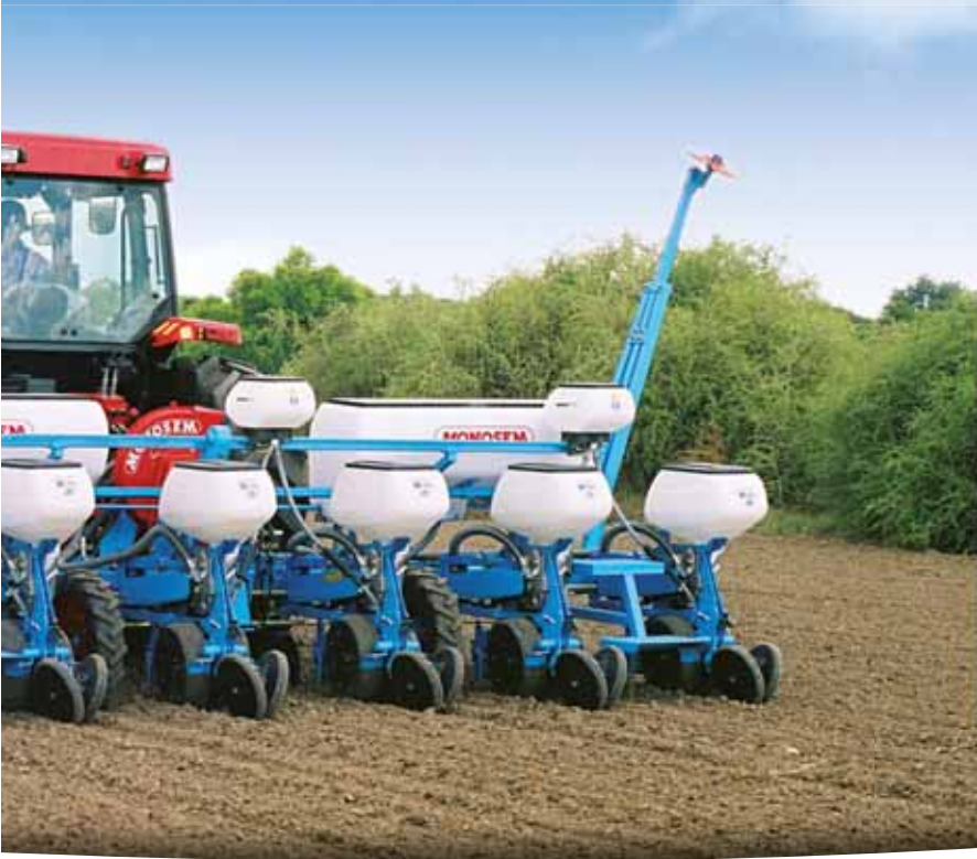
4-row rigid Monobar planter (75 cm inter row spacing)
