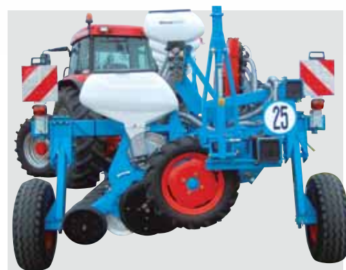
A transport carriage (lengthwise) is available for wide configuration planters. This transport carriage may be with manual or hydraulic lift.
