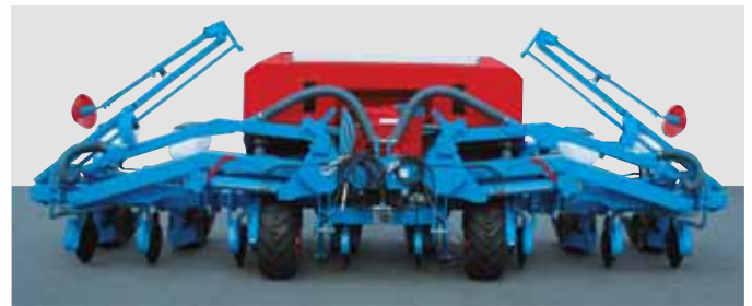
8-row rigid TFC folding planter (75 cm inter row spacing)
