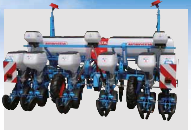
6-row Monoblock single telescopic planter (75 cm inter row spacing)
