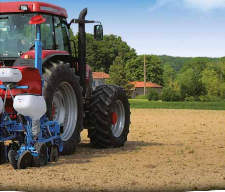
6-row Monoblock single telescopic planter (75 cm inter row spacing)
