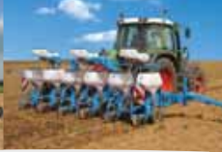
Special pneumatic « low-till » planter NX 2 with discs
