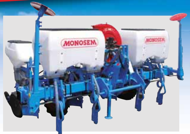
4-row rigid Monobar planter (75 cm inter row spacing)
