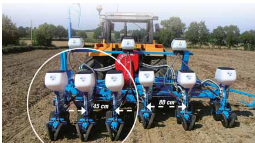
The 6-row Extend planter enables spacings of 45, 50, 55, 60, 65, 70, 75 and 80 cm.
