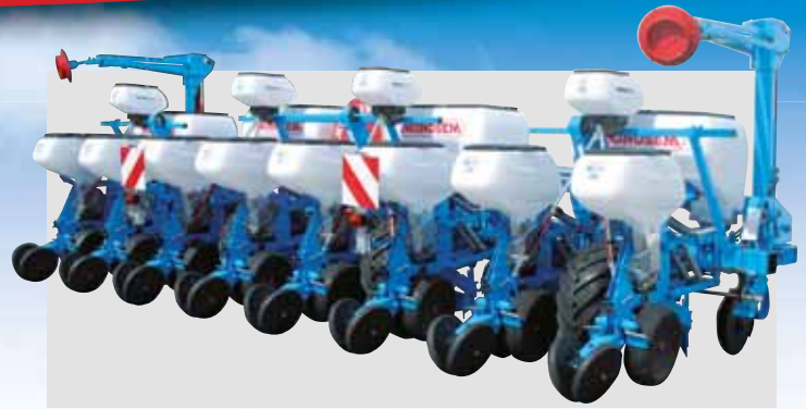
8-row Double bar folding planter (75 cm inter row spacing)
